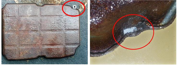
PML's design avoids the problems with the stock pan retaining clips. Bolts secure the pan to the transmission housing. PML pans do not use retaining clips.
