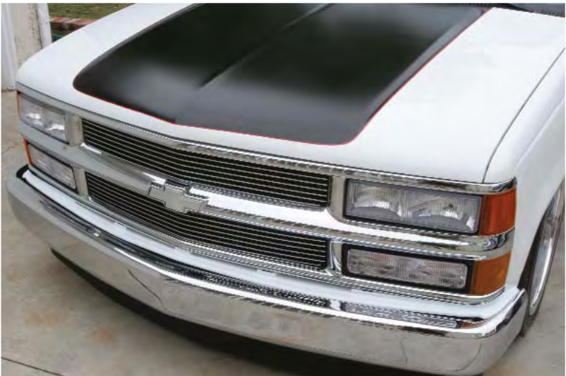
7. Tom McWeeney of Kustoms Inc. taped off the anti-glare shield on the hood and El Camino SS-inspired racing stripes that were hit with SEM Hot Rod Black.
