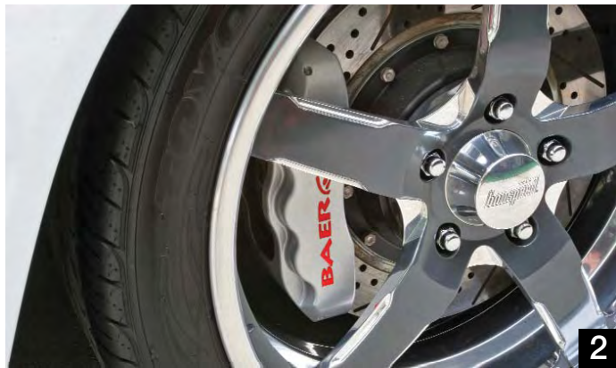
2. Twenty-inch bonspeed SS wheels were hit with sand-cast gray powder coating and wrapped in Toyo Proxes STII tires. Massive 14-inch rotors with six-piston Baer brakes bring them to a quick stop.
