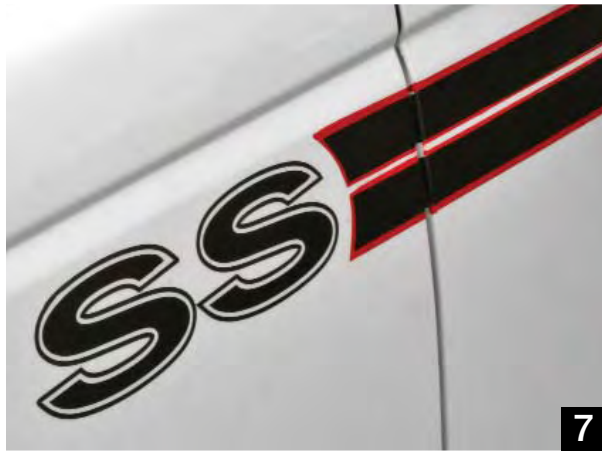
7. Tom McWeeney of Kustoms Inc. taped off the anti-glare shield on the hood and El Camino SS-inspired racing stripes that were hit with SEM Hot Rod Black.
