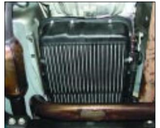
15. The PML transmission pan is set into place, bolted up, refilled with transmission fluid, and checked for leaks.
