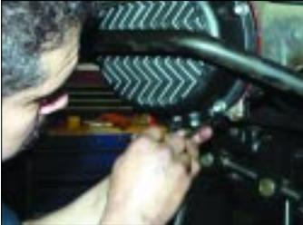
8. The new cover is bolted into place. After installation, the differential is refilled with gear oil and checked for leaks.
