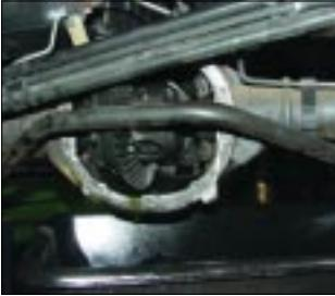
4. Once the stock cover is taken off and the old gasket material stripped away, the differential is ready to receive the new cover.
