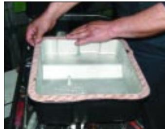
14. The gasket, supplied with the GM kit (which also includes the replacement filter) is positioned into place.
