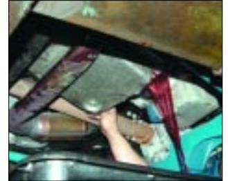
11. Once the pan is unbolted, transmission fluid is drained from the pan.
