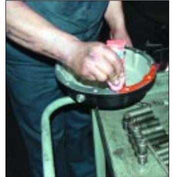
7. Sealant is applied to the inside flange of the PML cover to ensure a tight fit and no leaks.
