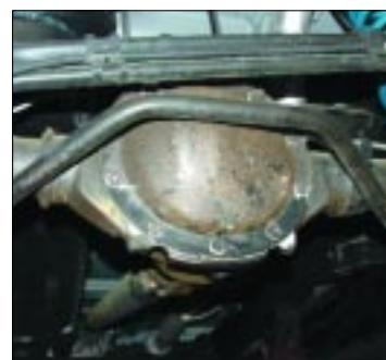
1. Here, the stock differential on the Avalanche is ready to be swapped out for an upgraded unit from PML.
