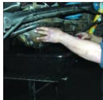
3. Draining the gear oil from the differential is a messy step in the install.
