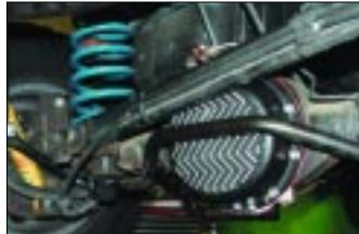
9. The PML cover sits proudly in place. One of the advantages of the new unit is that it uses a drain plug, so draining the oil no longer involves taking off the entire cover.
