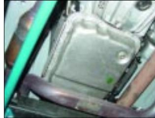
10. The stock transmission pan is much smaller and plainer looking than the PML piece that will replace the unit.
