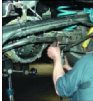
6. Since the PML cover is much thicker than stock, on our Avalanche application, the sway bar must be loosened and moved out of the way in order to install the new cover.
