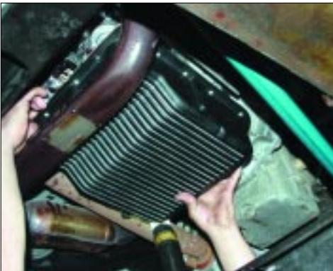
16. The new pan holds approximately 2 additional quarts of fluid and certainly looks a lot better than stock. After the install, the spilled and splattered fluid was cleaned with solvent, ensuring that smoking does not occur when the engine is started and parts heat up.
