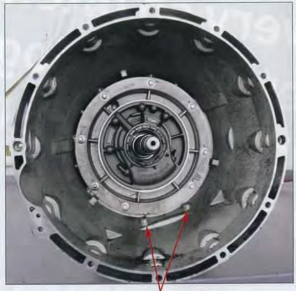
Front pan bolts are drilled through into bellhousing area
