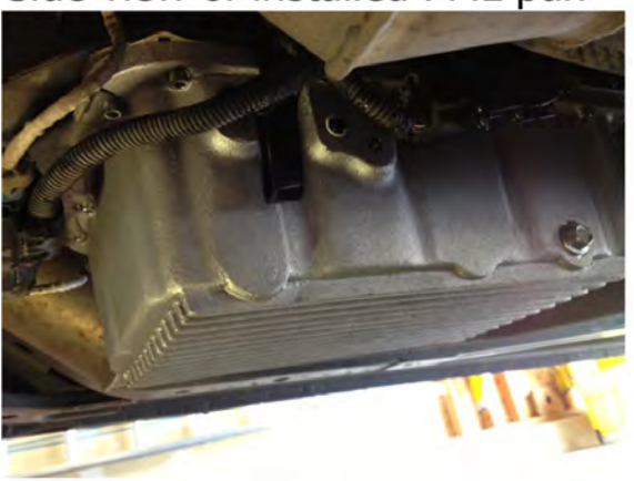
Side view of installed PML pan
