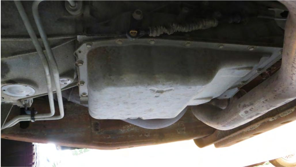
2. Allow 4 of the 18, 10 millimeter bolts to be removed to remain loosely in each corner, so the fluid can be allow to drain onto the oil drain pan below.
