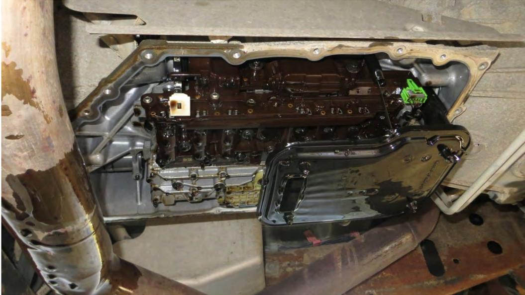
4. Clean the transmission mating surface; this is important to insure a leak free installation. I cleaned it with a rag; no abrasive material was used for this.
